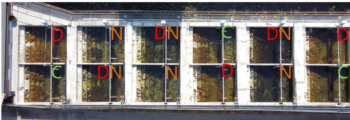
Figure 51 Overview of the 12 outdoor mesocosm basins at Solbergstrand, close to Oslo, Norway, including information of the design of the allocated treatments in this study, i.e. C-controls, N-nutrients, D-darkening, and the combination of darkening and nutrient enrichment (DN).
