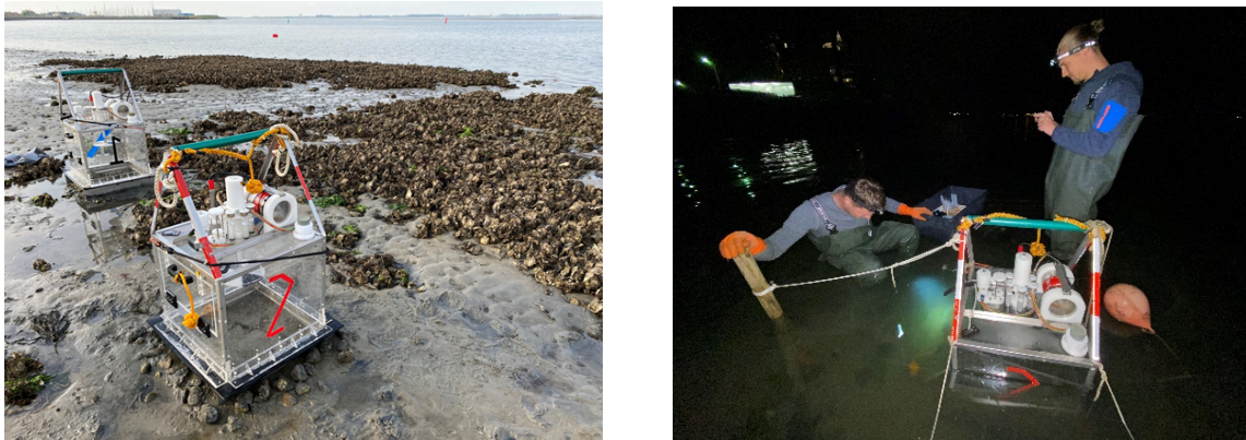
Figure 5: A. In-situ incubation apparatus used in FutureMARES to determine how oyster reefs impact the biogeochemistry (e.g. oxygen respiration rate) and the adjacent sediment and B. Incubation experiments on oyster reefs during the night. Credit: Brenda Walles
