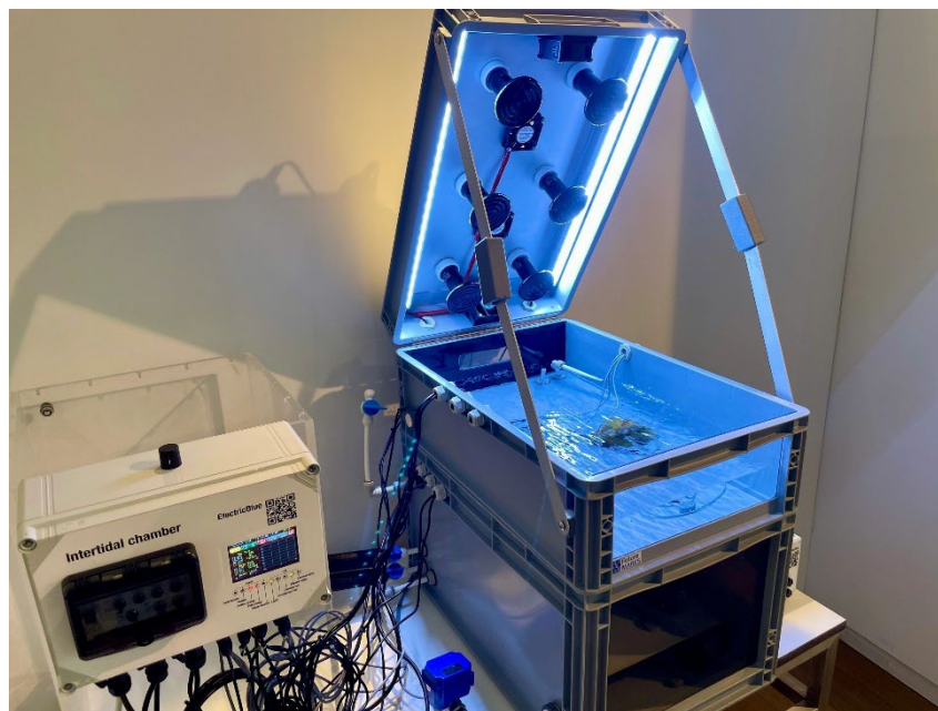
Figure 4: Intertidal chamber designed and partially funded within the WP3 -FutureMARES.
